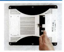
4 To connect the battery, the tab on the connector coming from the battery must snap over the tab on the wire coming from the tablet. Failure to connect the battery properly can result in fire and damage to the device. To disconnect a battery, hold the white plastic connecters at both sides with your fingers, press on the tab, and pull gently.
